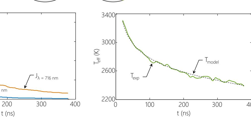
The above graphs show (left) the incandescence collected for Fe-Ar and (right) the experimental and modelled pyrometric effective temperature decay from those signals.
