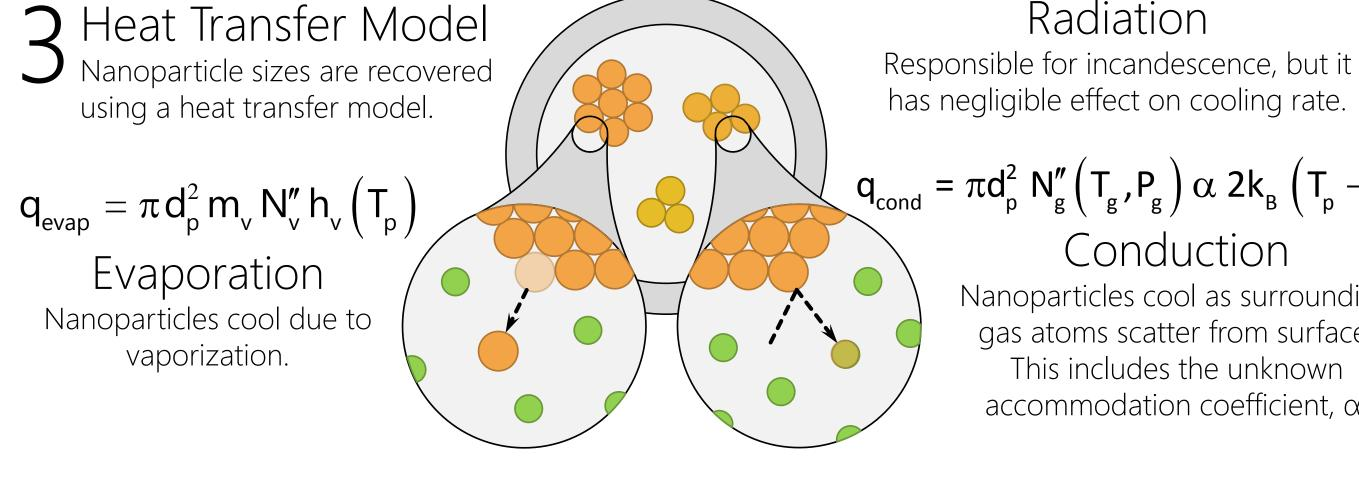
has negligible effect on cooling rate.  $q_{cond} = \pi d_p^2 N_g'' (T_g, P_g) \alpha 2k_B (T_p - T_g)$ Conduction
